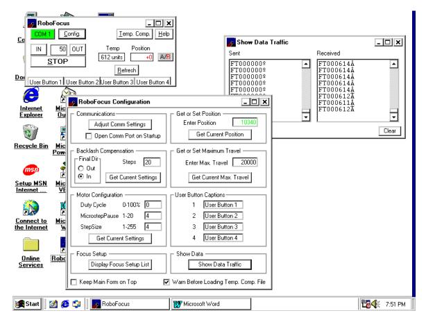
This is a typical screen shot showing the main RoboFocus window (upper left) that controls the system. The larger configuration window (lower left) is also shown. One of the options on the Configuration screen is the ShowData window, shown open on the upper right (this shows the data traffic to and from the roboFocus controller.
