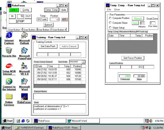
Note: temperature is measured using the built in temperature sensor in the RoboFocus controller. The temperature readings are in raw temperature counts (the counts are close to twice the absolute temperature in deg. Kelvin, with 32F=0C=273K=546 counts approximately), or in F, or C.
