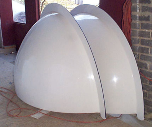
Two dome halves, slot edges up
